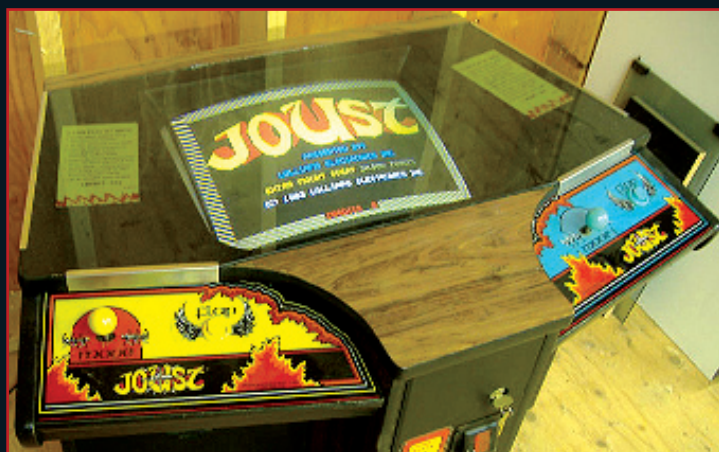
» The rare cocktail version of Joust . "This was a lot of effort for little return," says John. "Cocktail cabinet sales at all coin-op manufacturers were falling off, so the demand was low. It had to fit two people on the same side – in most table games, players took turns so the software had to flip the screen. Our advantage was we could use the exact same ROMs for either cabinet."
